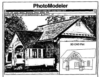
PhotoModeler™ produces 3D models from photographs. The models are accurate and detailed and the process is organized and easy to learn. The models can be exported as 3D DXF files and imported by most CAD, animation and rendering programs. Documenting cultural resources and gathering stratigraphic data are potential applications. PhotoModeler runs under Windows 3.1 and sells for \$895. A working, limited-function version with a tutorial is available for \$25.
