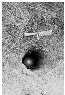
Figure 2: View of a cyberstake or ball marker in auger hole.
