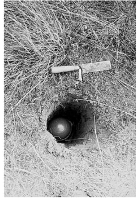
*Figure 2: View of a cyberstake or ball marker in auger hole.*
